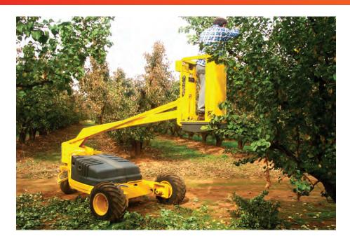
Powerladders produced by edp Australia have helped growers improve efficiency and reduce the risk of injury in orchards for over 30 years. Powerladders are known more formally as Mobile Elevating Work Platforms (MEWPs).
