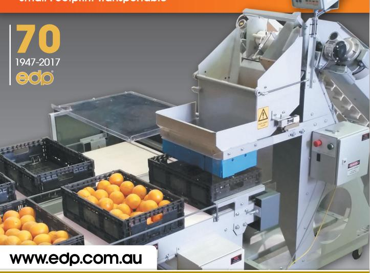
The **edp Minibagger** has become very versatile. The hopper accumulates the pre-batched weighed product ready for discharge. An infeed and exit system automatically indexes crates or cartons for filling. This provides a totally automatic packaging solution. The minibagger's weight program can be altered in seconds, making this Minibagger exceptionally user friendly.
