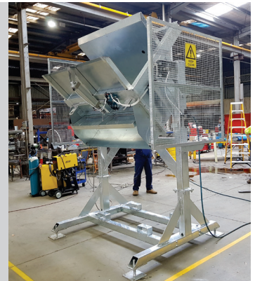
Optional Hot Dipped Galvanized bin tipper in the tip position.
